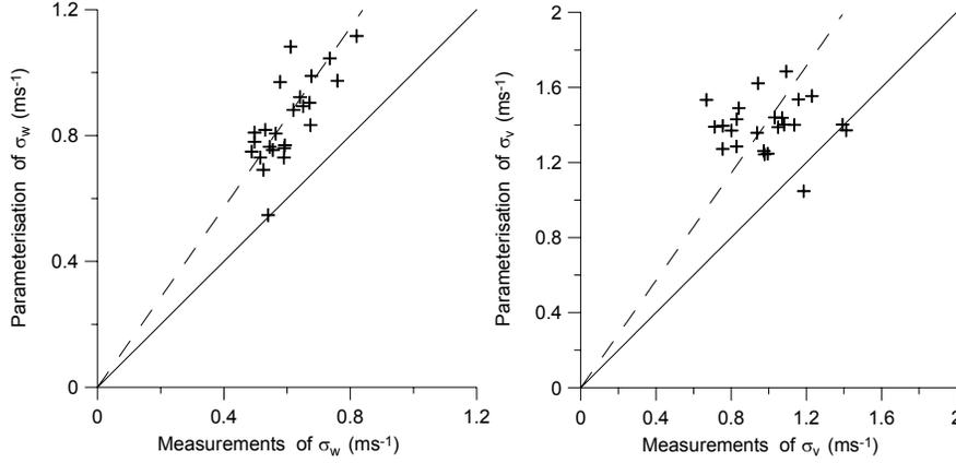
**Figure 4.** Observed half-hourly averaged versus parameterisations of  $\sigma_w$  (left panel) and  $\sigma_v$  (right panel).
