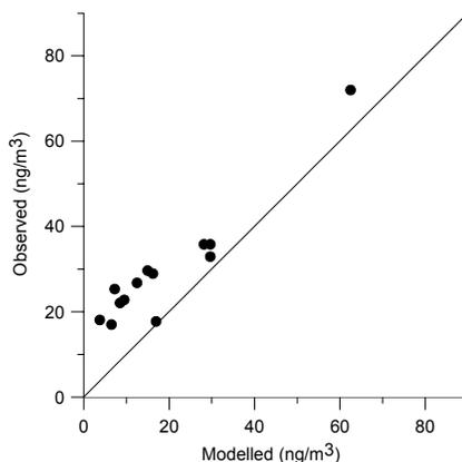
**Figure 6.** Observed and modeled near-roof concentrations at the 13 tracer sampling sites for the experiment of June 26 2002. Meteorological input data to the model are three-hourly averages and so are the observed concentrations. Parameterizations for the turbulence profiles are employed.
