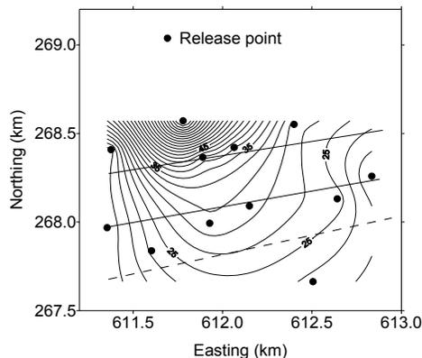
**Figure 2.** Isolines of interpolated tracer concentrations [ $\text{ng m}^{-3}$ ] averaged over the period for the experiment on 26 June, 13-16 CET. The filled circles designate the tracer release and sampling positions. The full lines represent crosswind profiles that formed the basis for the estimation of  $\sigma_y$ , see Table 1. The profile along the dashed line was not used due to insufficient data coverage. The co-ordinate system as in Figure 1.
