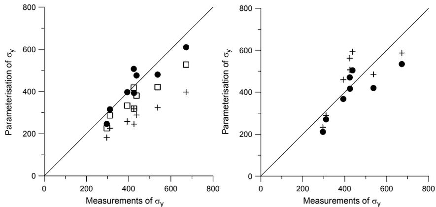
**Figure 5.** Measured and modelled values of  $\sigma_y$ . . In the left panel the simulations are performed using observed values of  $\sigma_v$  and for  $T_y = 200$  s (+);  $T_y = 600$  s (□) and  $T_y = z_i / \sigma_v$  (●). In the right panel the simulations performed by use of parameterised values of  $\sigma_v$  and  $T_y = z_i / \sigma_v$  (●). Also the fully empirical parameterisation based on  $X$  is shown (+).
