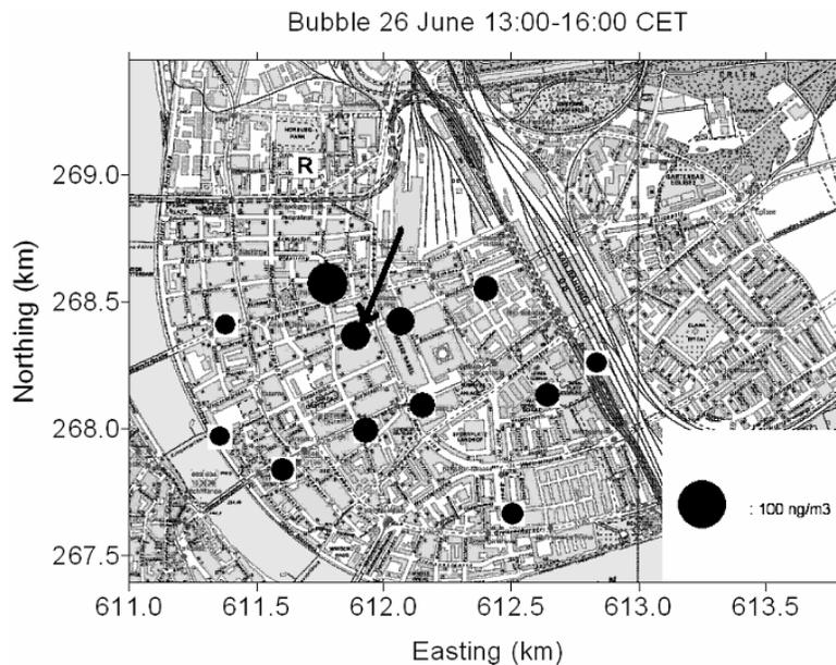
**Figure 1.** The tracer concentrations on 26 June, 13-16 CET. The release point is marked with R; at the tracer sampling positions the measured concentration is indicated with the area of the filled circle. For comparison a filled circle representing  $100 \text{ ng m}^{-3}$  is shown in the white box. The arrow shows the position of Sperrstrasse. Base map (c) copyright GVA BS, 25.10.2002.
