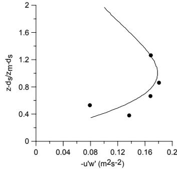
**Figure 3.** Profile of observed (filled circles) and fitted (full line) Reynolds stress component  $-\overline{u'w'}$  at Sperrstrasse during the tracer experiment on 4 July. The displacement height is  $d_s$ .
