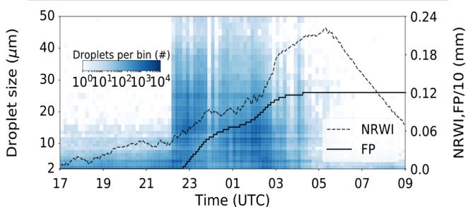
Fig 3: Example of DSD (blue), fog precipitation from fog collector (black solid) and non-rainfall water input from microlysimeters (black dashed) during a fog event in Gobabeb (27-28.9.2017). Note that FP is scaled down.
