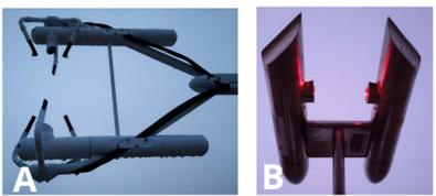
Fig 2: Sonic anemometer (IRGASON, A) and cloud droplet probe (CDP, B).
